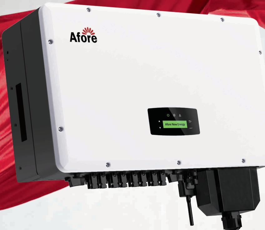
The Afore BNT Series Three-phase string inverters are designed for commercial and power plant PV system applications, rating from 17kW to 30kW. All models with aluminum housings which is anodized, increasing durability and effectively prevents corrosion. Equipped with external inductors, ensure efficient heat dissipation, which significantly improves the reliability and extends the life of the inverters.
