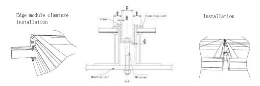
outside,1 Different models of assembly and installation sizes of fixture
